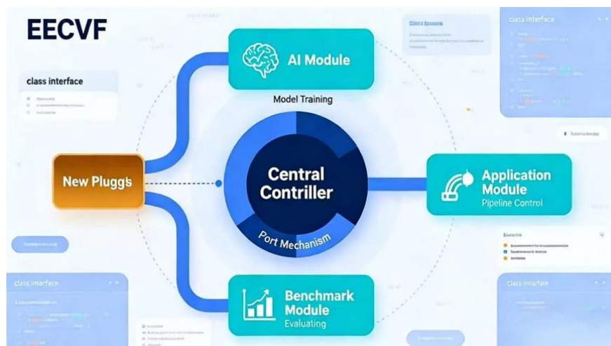
Figure 2. Centralized Structure of EECVF. In this figure, it shows that the centralized controller links the intelligent algorithm part (model learning) how these modules are connected to each other, i.e., application module (pipeline control), benchmark module (evaluation) via the port mechanism; and how a new plugin is able to mount on the system.
